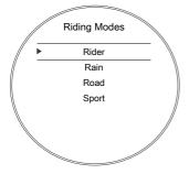
Push the joystick down/up until the required setting option is selected and press the joystick center to confirm
