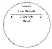
To adjust the engine speed threshold (RPM) for the gear shift indicator:
