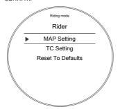
Push the joystick down/up until the required option is selected and press the joystick center to confirm.
