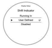
The engine speed threshold can be defined and reset, and the gear shift indicator can be disabled. Once the engine has been broken in (at 1,000 miles), the Running In option is replaced with a Default option.
