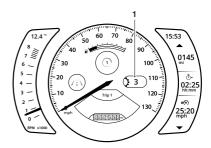
1. Gear position display (third gear shown)
