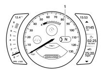
Gear position display (neutral position shown)
