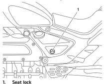
The seat can be removed to gain access to the battery, fuses, storage compartment and USB socket.
