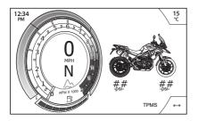
The front or rear tyre will be highlighted on the motorcycle image to indicate that the tyre pressure is below the recommended pressure.
