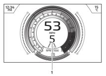
1. Gear position display (fifth gear shown)
