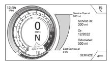
The service interval shows the distance and date that the service is required to be completed by.
