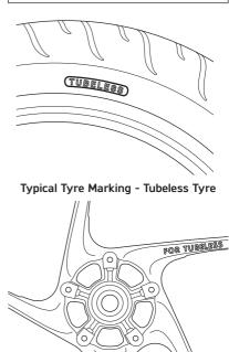
Typical Wheel Marking - Tubeless Tyre
