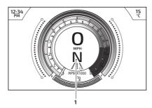
1. Gear position display (neutral position shown)
