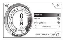
The engine speed threshold can be defined and the gear shift indicator can be disabled. Once the engine has been run in (at 1,000 miles), the Running In option is replaced with a Default option.
