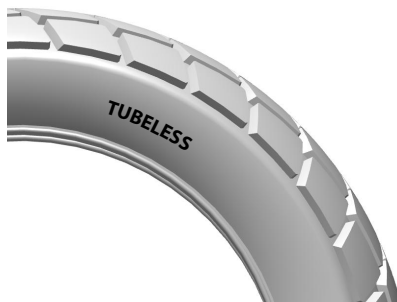
Typical Tire Marking - Tubeless Tire
